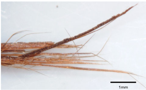
Fig. 5 Rupture point of bamboo fiber
